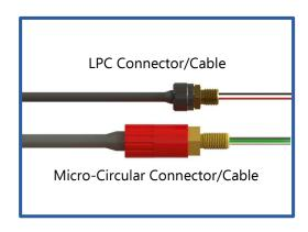
The LPC bulkhead connector fits in a standard 7/16"-20 threaded hole (or in a 7/16" thru-hole if using the included nut), and is available in 3-pin and 6-pin versions. It can be installed in the wall of any enclosure, provided that the enclosure has a smooth outer surface to seal against the connector's O ring. LPC cables also come in 3-conductor or 6-conductor versions and 1-meter or 2-meter lengths.
