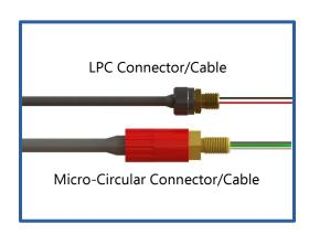
The LPC bulkhead connector fits in a standard 7/16"-20 threaded hole (or in a 7/16" thru-hole if using the included nut), and is available in a 3-pin version. It can be installed in the wall of any enclosure, provided that the enclosure has a smooth outer surface to seal against the connector's O ring. LPC cables come in 1-meter or 2-meter lengths.
